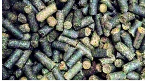
Fig. 4. The upgraded pine waste after thermal pre-treatment
